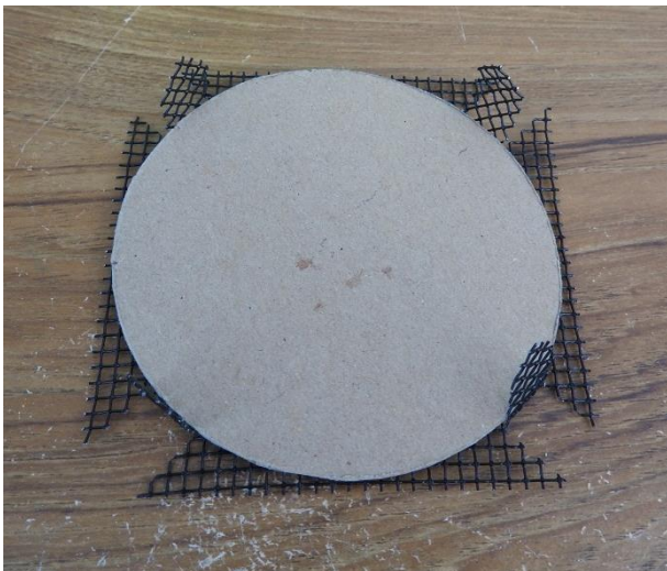
Fig. 3 Forming the corner tabs
